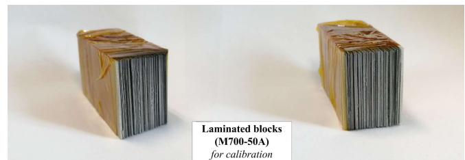
Fig. 24. Blocks of standard laminated electrical steel for the calibration of the U-shape tester.
