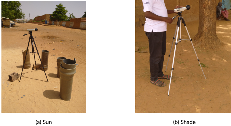
FIGURE 2 Heat stress data logger setup.
