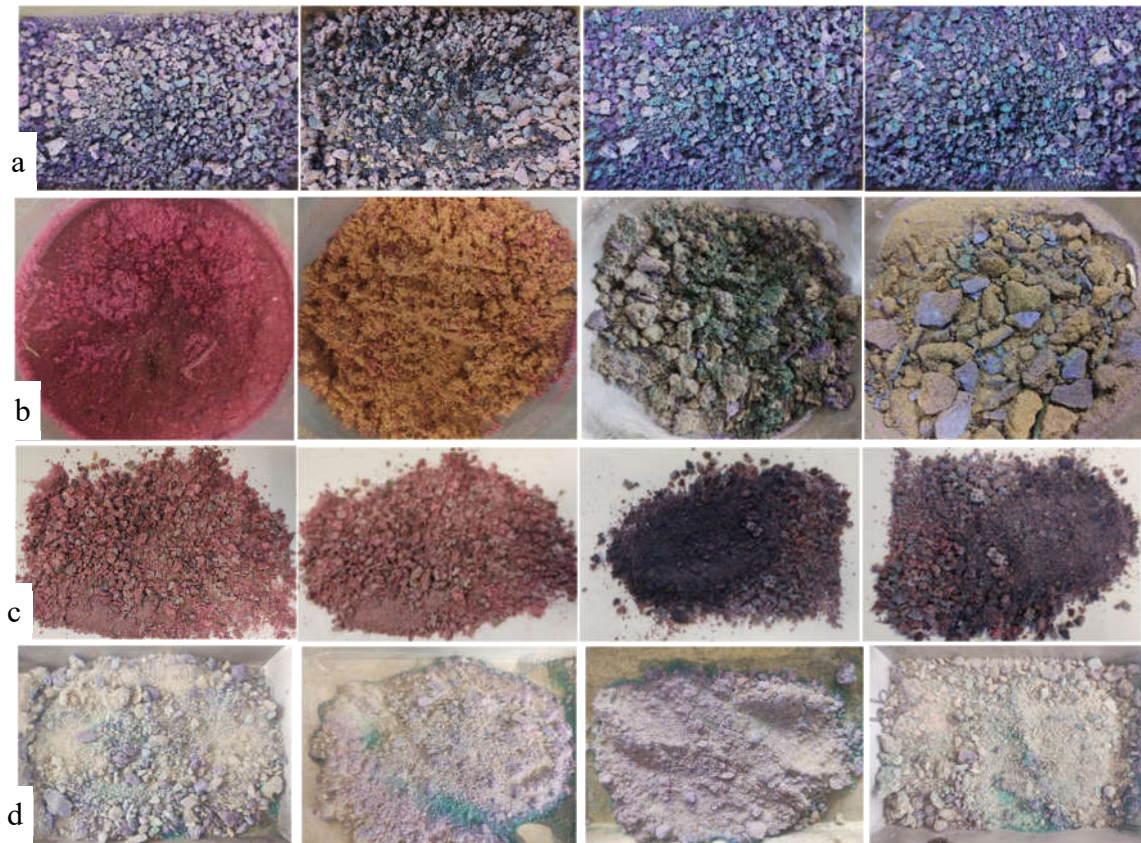
Figure 6. Colored aggregate samples for the colorimetric method for a) FRL, b) SS, c) FRP and d) MQS
