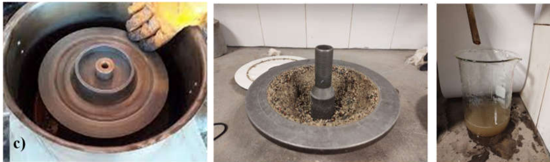
Figure 9. a) Moisture-time curve for the horizontal bowl centrifugal method, b) correlation with the cone shape in the cone method and c) Centrifugal set and water recovery
