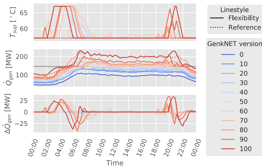
Figure 9. For the Winter_Large \Delta p_e day, the results of the base-peak plant optimisation for the 11 selected GenkNET versions with a base load ratio of 95 % are shown. From top to bottom, the supply temperature at the plant, the heat injection and the heat injection response are shown. In the middle graph, the maximum heat output of the base unit is indicated by the grey horizontal line.
